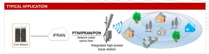
In rural and suburban areas, the wireless network coverage is relatively wide, but the users are less fixed than the fixed ones. By deploying LTE integrated high-power base stations in a town or natural village, the signal coverage in a small area can be achieved, reaching low Investment in rural 4G wireless access.
